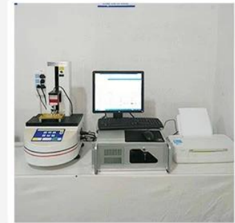
3. Load Curve Meter
