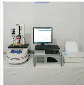
3. Load Curve Meter
