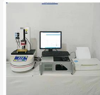
3. Load Curve Meter
