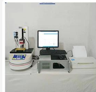
3. Load Curve Meter
