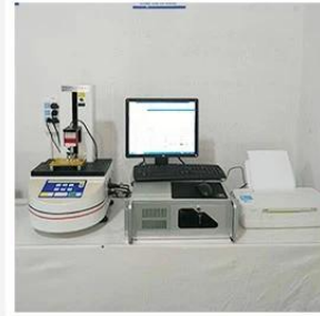
3. Load Curve Meter
