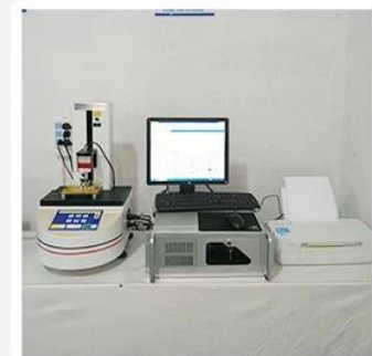
3. Load Curve Meter
