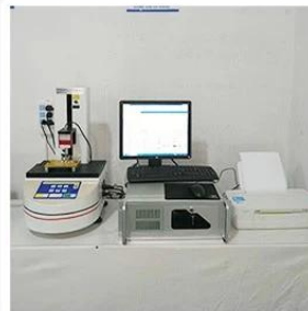
3. Load Curve Meter
