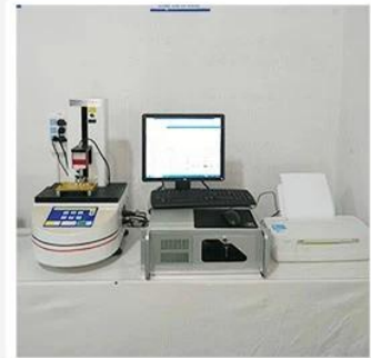
3. Load Curve Meter
