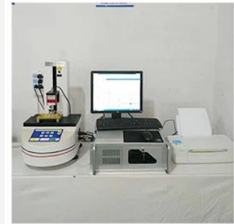
3. Load Curve Meter
