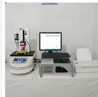
3. Load Curve Meter
