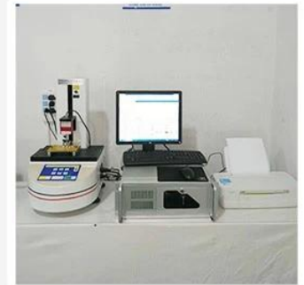
3. Load Curve Meter
