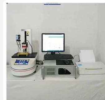
3. Load Curve Meter
