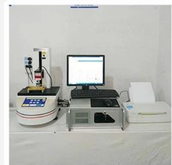
3. Load Curve Meter
