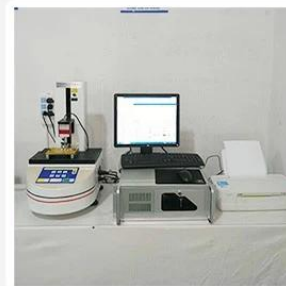
3. Load Curve Meter
