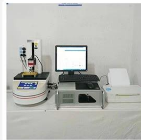
3. Load Curve Meter
