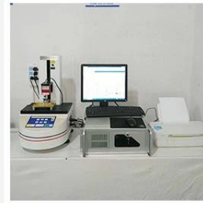
3. Load Curve Meter
