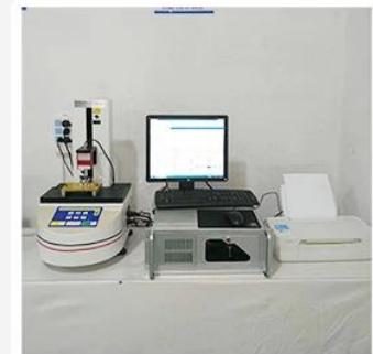
3. Load Curve Meter
