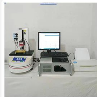
3. Load Curve Meter
