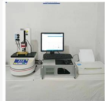
3. Load Curve Meter
