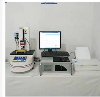
3. Load Curve Meter
