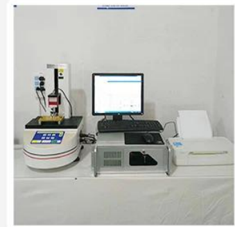
3. Load Curve Meter
