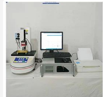
3. Load Curve Meter
