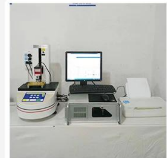
3. Load Curve Meter
