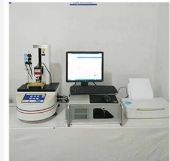
3. Load Curve Meter
