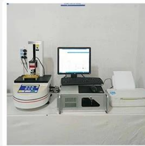
3. Load Curve Meter
