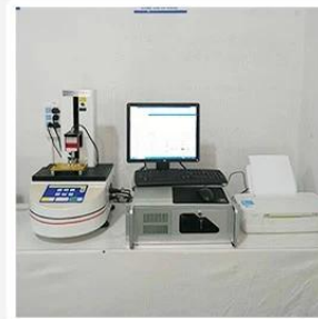
3. Load Curve Meter
