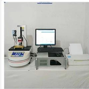
3. Load Curve Meter
