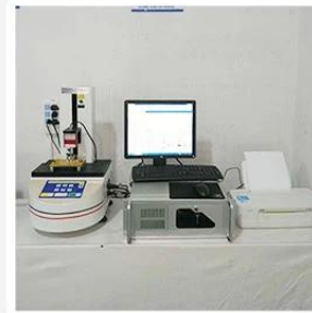
3. Load Curve Meter
