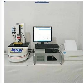
3. Load Curve Meter
