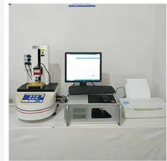
3. Load Curve Meter
