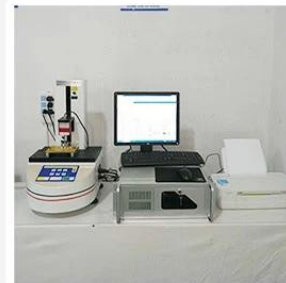
3. Load Curve Meter
