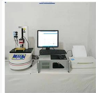
3. Load Curve Meter
