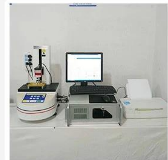
3. Load Curve Meter
