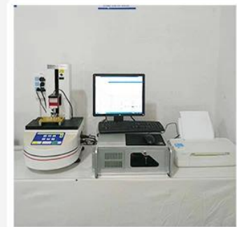
3.Load Curve Meter
