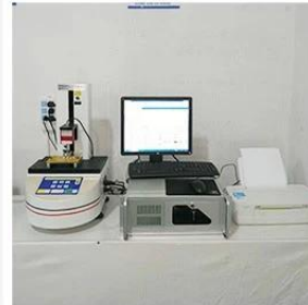
3. Load Curve Meter
