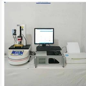
3. Load Curve Meter
