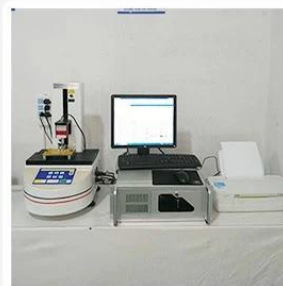
3. Load Curve Meter
