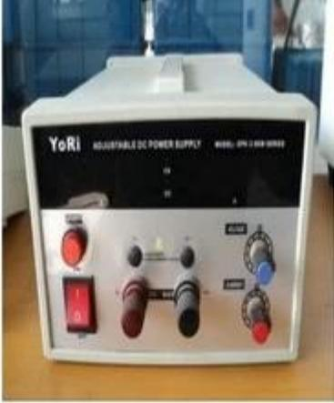
A white, rectangular DC power supply unit with a black front panel. It features a red power switch, several output terminals, and a digital display. |
