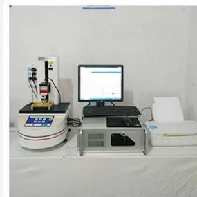
3. Load Curve Meter
