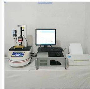
3. Load Curve Meter
