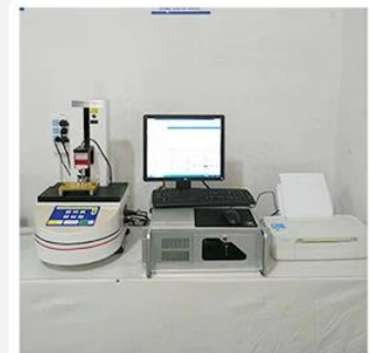
3. Load Curve Meter
