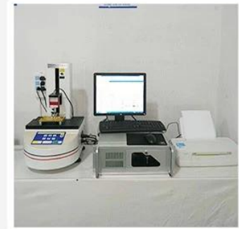
3. Load Curve Meter
