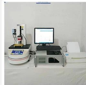
3. Load Curve Meter
