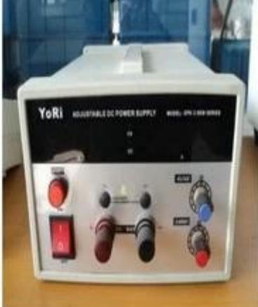
A white, rectangular power supply unit with a black front panel. It features a red power switch, several control knobs, and output terminals. |
