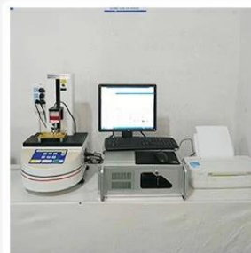
3. Load Curve Meter
