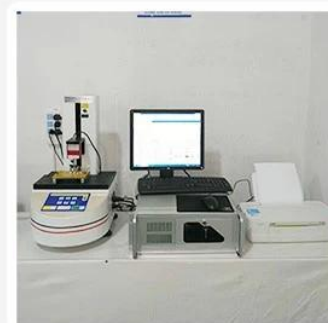
3. Load Curve Meter
