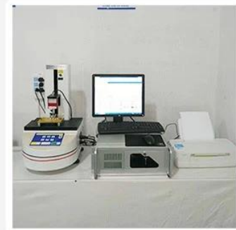
3. Load Curve Meter
