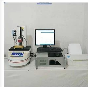
3. Load Curve Meter
