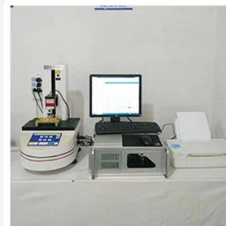
3. Load Curve Meter
