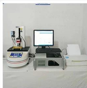
3. Load Curve Meter
